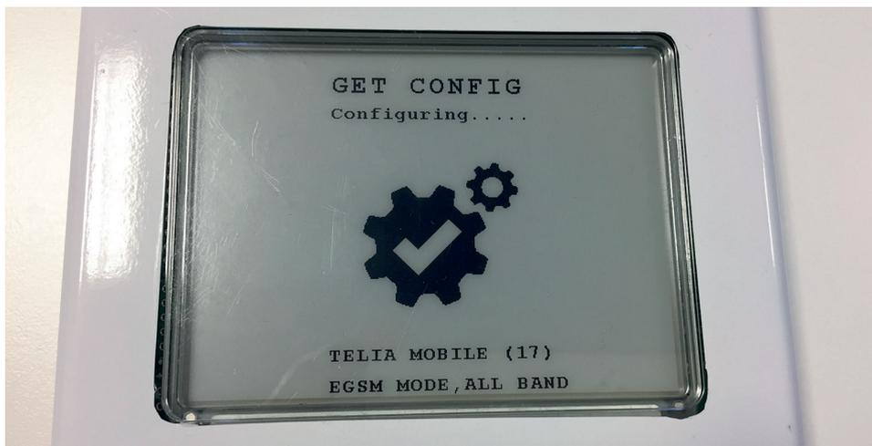
Step 4: The Qlvr Box will configure automatically and upon completion, display the current time for about 8 seconds. After that, a beep will be heard, and the Qlvr Box will display the last employee card registration time.
